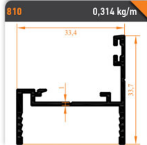
810 0,314 kg/m Sabit Cam Kilit Profili Constant Glass Lock Profile
