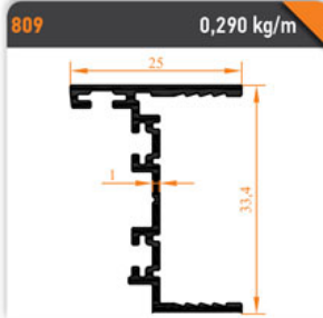
809 0,290 kg/m Sabit Cam Menteşe Profili Constant Glass Hinge Profile
